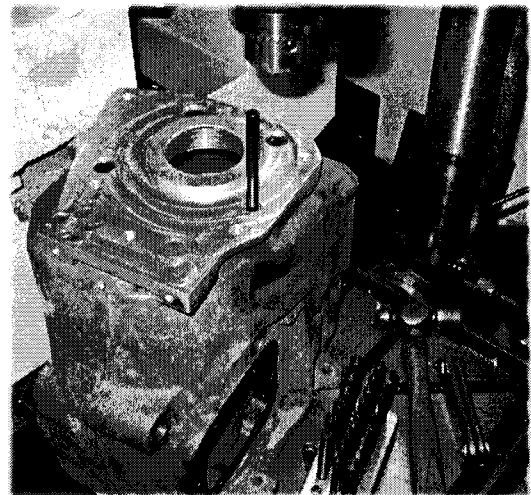
If available, the use of a transfer punch will help start a precise bore.
